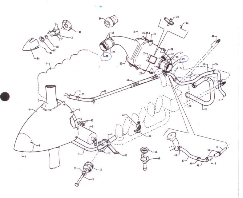
Figure 54 Power Plant Installation
