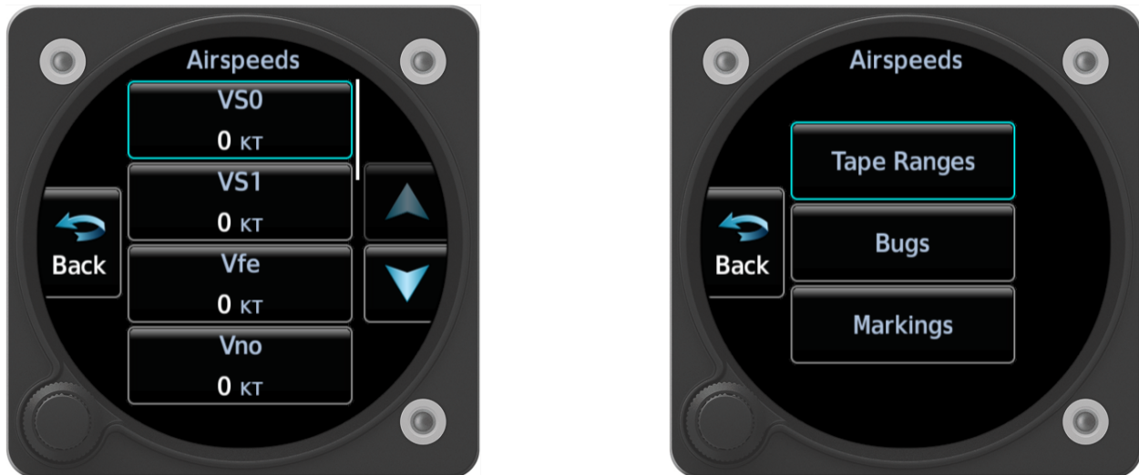
Figure 4-7 Basic (Left) and Advanced (Right) Airspeed Configuration Type Settings
